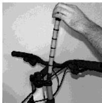
*Removing Spring Stack*
