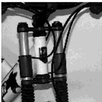
**Proper Cable Routing**
