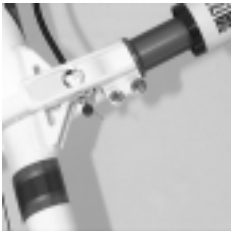
Lockout switch in open / unlocked position
